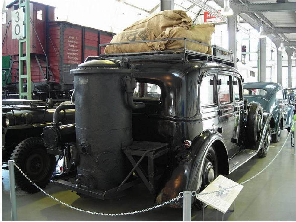
Chart 1 cars use wood gasification equipment and gas engine
